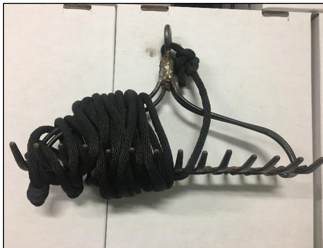
Double-headed, weighted garden rake, attached to a rope used to survey aquatic vegetation.
