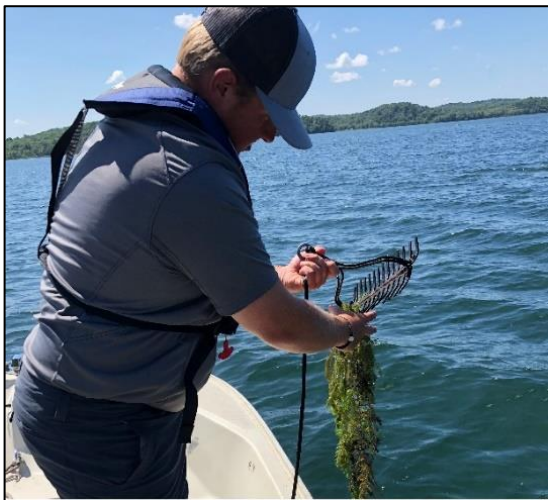
Double-headed, weighted garden rake, attached to a rope used to survey aquatic vegetation.
